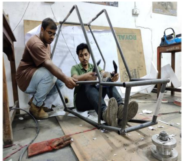
Roll cage with Metal Tubes
